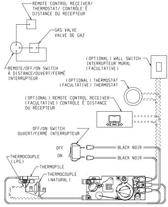
IF ANY OF THE ORIGIONAL WIRE AS SUPPLIED WITH THIS UNIT MUST BE REPLACED. IT MUST BE REPLACED WITH NO. 18, 150°C WIRE OR ITS EQUIVALENT.
